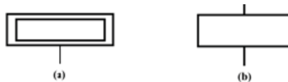
Fig. 21.4 An initial step (a) and a regular step (b) in an SFC
