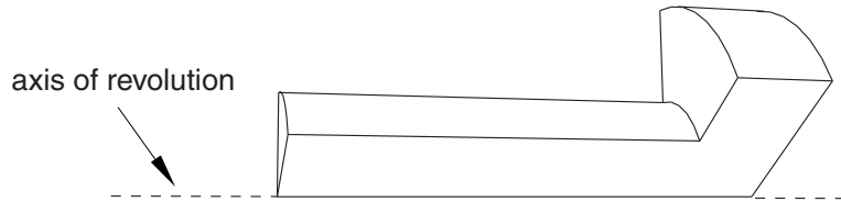
Figure 17–76 Abaqus/CAE cannot mesh a region with hexahedral elements if one or more edges lie along the axis of revolution.
