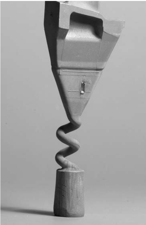
Fig. 3.6. Details of the starter block and pig-tail grain selector from the Trent 800 high-pressure turbine blade casting.
