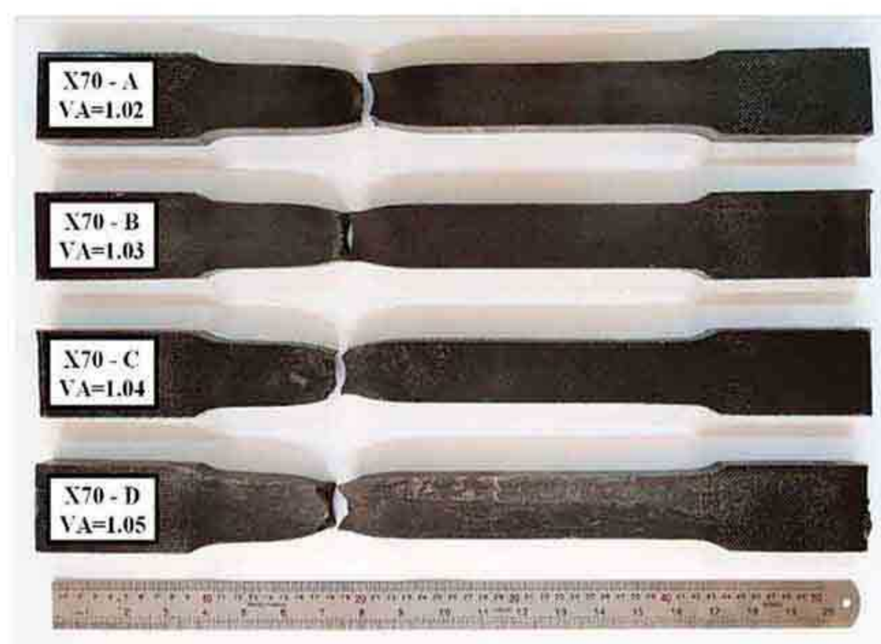
Fig. 15 X70 samples of tensile test.
