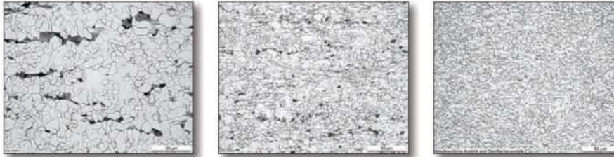
Fig 2 Effect of cooling rate on microstructure of X65 linepipe grade
